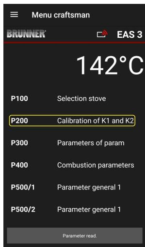
Press the button **Calibration of K1 and K2** to open the **P200 Menu** allowing for the calibration of motors.
