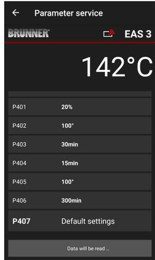
The parameters of combustion process can be reset to initial values by clicking **P407 Default settings**.
