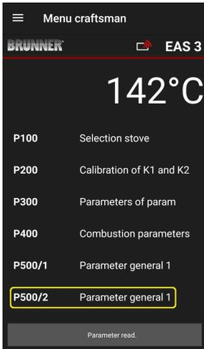
In this menu you can set the General parameters' part 2 (P513 – P517). The value ranges are shown in the *programming instructions* (chapter *General parameters*).
