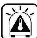
The combustion chamber temperature is above the allowed maximum for the stove or fireplace type.
