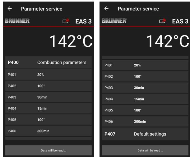
The parameters of combustion process can be reset to initial values by clicking **P407 Default settings**.
