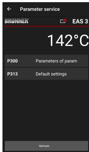
Under **P300 Heater parameters**, after automatic transmission of data, the current values for each parameter of the selected heater type are shown.
