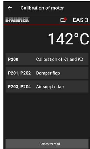
Click on **Start P201** → motor opens to 100%, if not open yet, then moves back to 0%. Now it is possible to start the manual calibration. Press **+** or **-**.
