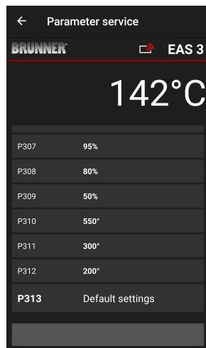
The heater parameters can be reset to initial values by clicking **Factory defaults**. The pop-up menu must be confirmed by selecting **Reset now**.
