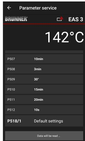
The parameters of combustion process can be reset to initial values by clicking **Default settings**. The pop-up menu must be confirmed by selecting **Reset now**.
