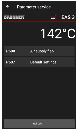
Under **P600 Damper flap K2**, after automatic transmission of data, the current values for each parameter are shown:
